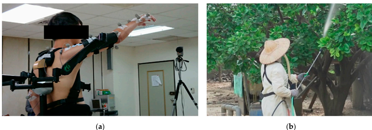
Figure 1. Experimental photographs. (a) Photograph of the passive upper-limb exoskeleton (PULE) during the simulation of fruit thinning; (b) Photograph of the pesticide spraying activity of the pomelo tree.
