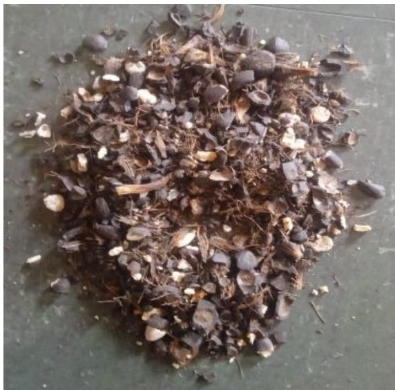
4(a). The cracked kernel shells using the 3-arm hammer beater awaiting sorting
