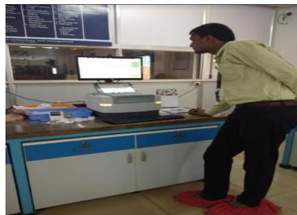
Fig. 2. The X-Ray fluorescent spectrometer for chemical analysis (Make: PANalytical B.V.)
