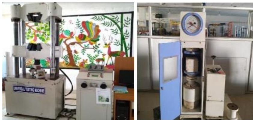
Fig. 4. The UTM and Digital concrete testing and DCTM used for testing the samples
