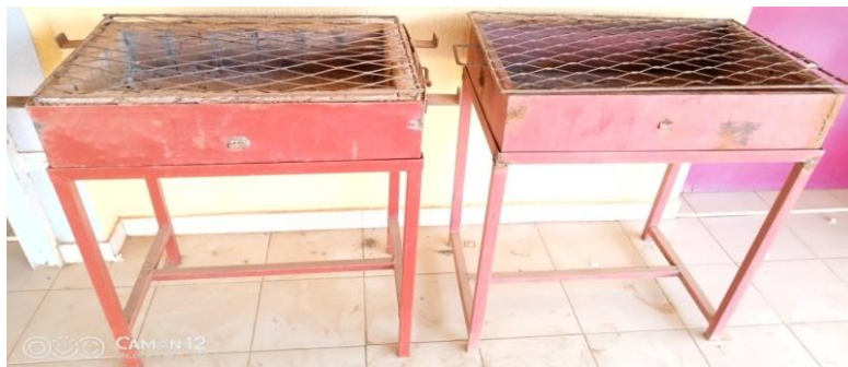
Fig. 1. Insulated oven (left) and non-insulated oven (right)
