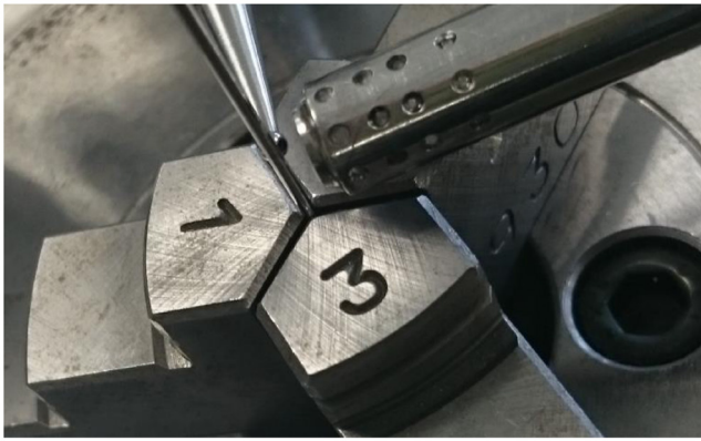
Figure 3. Chromatic confocal sensor versus contact measurement on a 1 mm diameter cylinder gage (top-down view).
