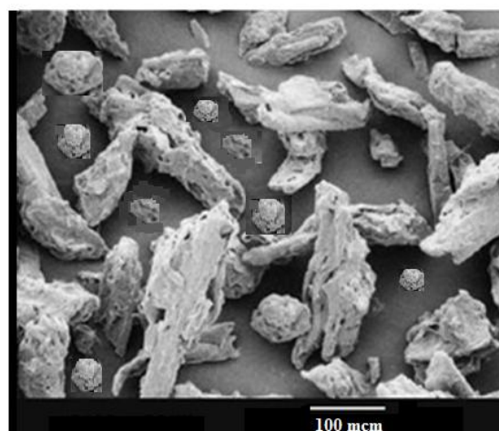
Fig. 2. SEM image of composite containing aggregates of rod-like microparticles of biomass and round microparticles of INOS
